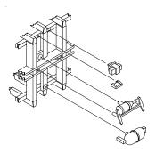
**Step (2).** Choose either an X2F coupler (PN0018) or Accumate coupler (PN0120), and place it into the coupler box (PN0019). Install the coupler lid (PN0020), and attach the assembly to the underframe (PN0369) using the short screw (PN0100).
